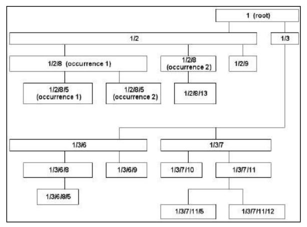
Each cell in the diagram represents an element whose tagPath is indicated within the cell. The numbers within the tagPath are tagValues; for simplicity, tagTypes are omitted, and assumed all to be the same. Leaf-nodes are highlighted by double-lined cells.
